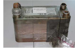
Fig. 3 Failed plates heat exchanger
